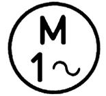
BAUER geared motors for operation on a single-phase AC power supply are supplied with specially adapted asynchronous motors with hysteresis circuit. By the use of special design features and, in some cases, alloy rotors, a starting torque that is only marginally below the rated torque is produced without the need for additional starting aids.
